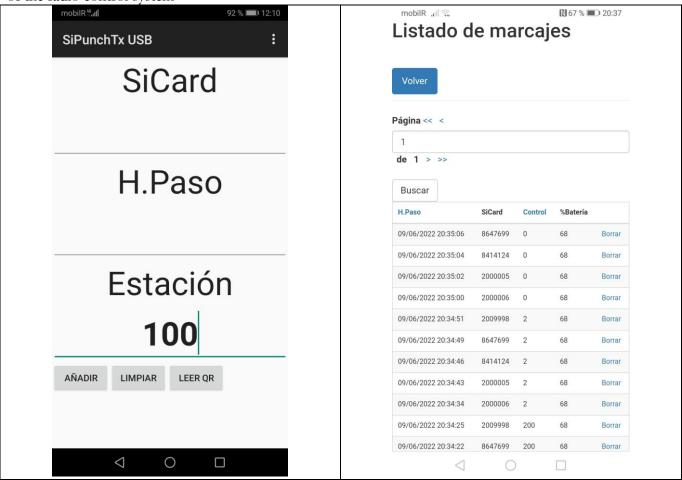
With NFC activated on the Smartphone, simply bring an NFC card close to the device (usually at the top) and the reading process will be activated. If it is the definition of a station, for example Control:100, the result will be that the received value will be written in the station field, but no reading will be sent.
